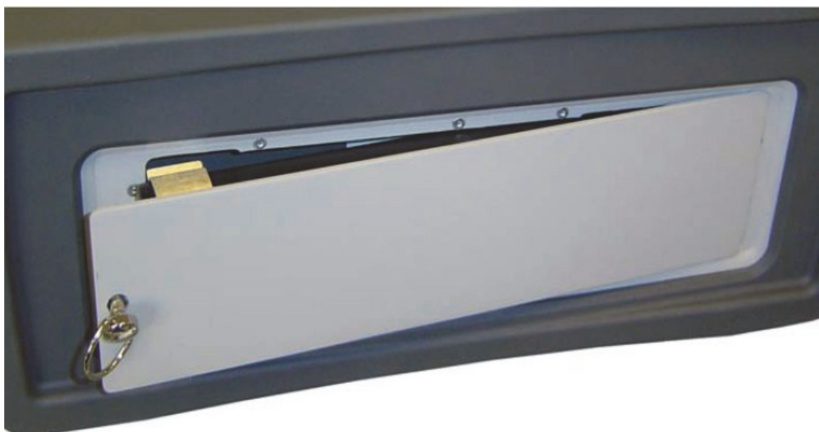
Figure 4-2. Opening the Battery Access Door
