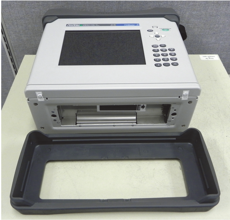
Figure 5-13. Remove the Bottom Bumper
