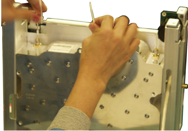
Figure 5-38. Tie Wrapping Cables for Option 700
