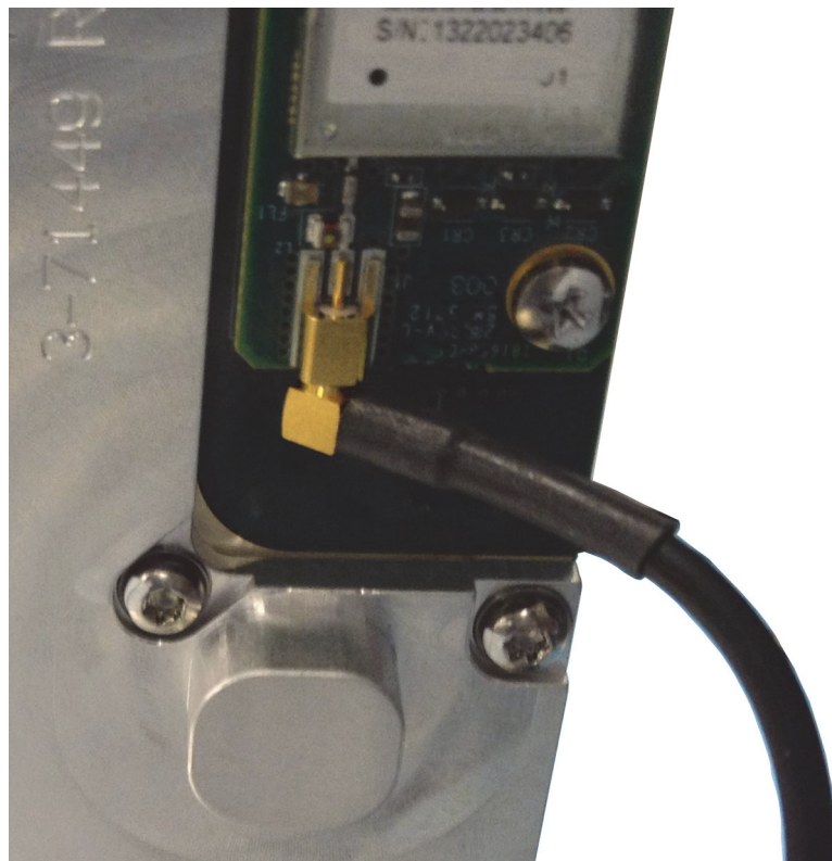
Figure 5-40. GPS Module with MMCX Cable Attached
