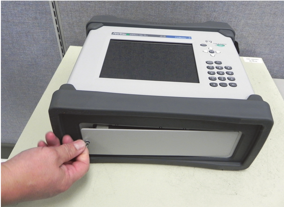
Figure 5-12. Remove Battery Door
