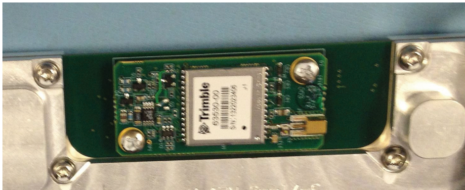
Figure 5-39. GPS Module (Option 31) on Motherboard
